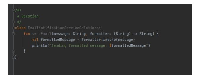
This time, we made the EmailNotificationService independent of the formatter implementation. The only thing that this service care about is that the formatter has to return a String value. As we can see, applying this principle gives us much more flexibility.
